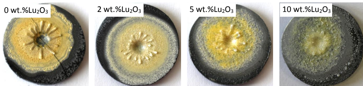
The surface of ZrB_2 -SiC samples with different amounts of Lu_2O_3 after the ablation test at the temperature of 2600°C for 60 seconds.
